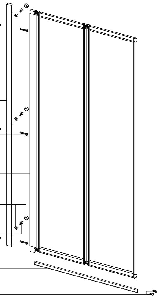
PRE-INSTALLED VERTICAL SEALS FOR DUO / JOINTS VERTICAUX
